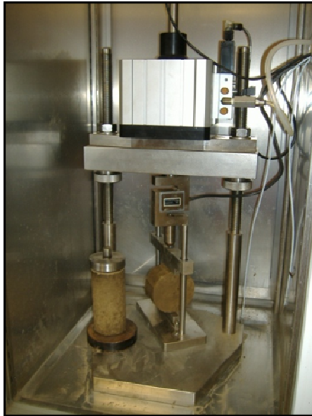
(a) Servo-pneumatic test set-up
