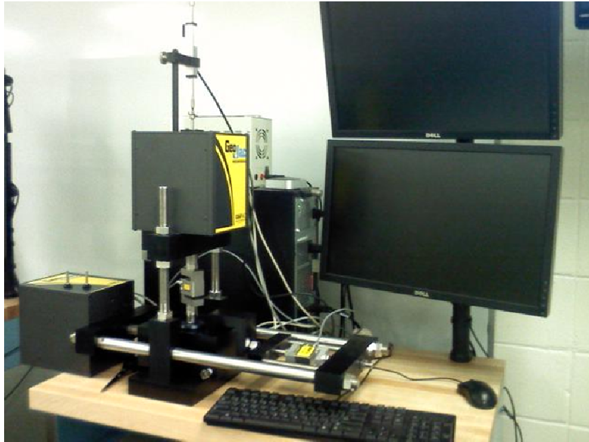
Figure 4.6: GeoTAC DigiShear direct shear apparatus
