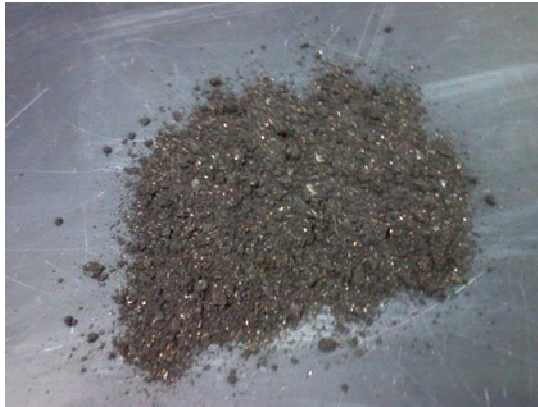
Figure 4.11: Recycled asphalt shingles
